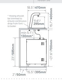
• This equipment must be installed with adequate backflow protection to comply with all applicable federal, state and local codes.
